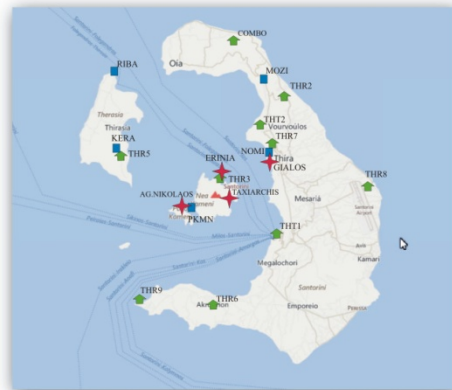
Figure 7. Main monitoring networks of the Santorini volcano, currently operated with the support of ISMOSAV (Seismograph: greens lodges, Tide Gauge-Temperature Measurement: red stars, Geodetic-GPS Stations: blue squares).
