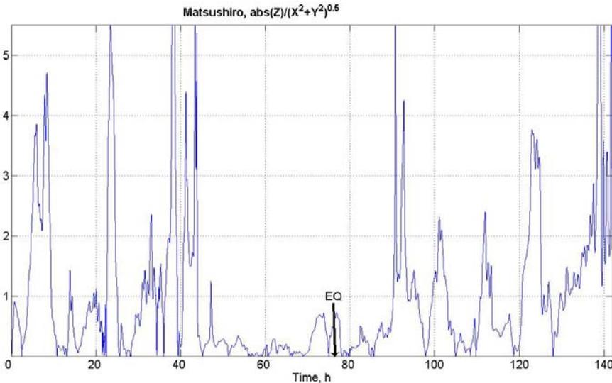
**Figure 4** The ratio  $Z/(X^2+Y^2)^{0.5}$  for pre-EQ ULF magnetic field near Matsushiro site is shown, where X, Y, Z are the components of magnetic field; abscissa is the local time of June 28, 1998.
