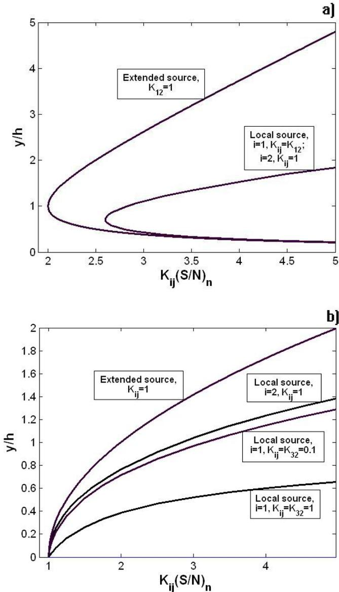
**Figure 2** The normalized distance against normalized signal to noise ratio for both local and extended sources of anomalous magnetic field signals: a) for vertical component; b) for horizontal components.
