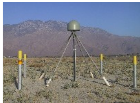
Figure 2. The deep drilled brace
